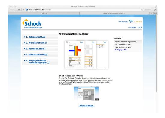
Based on the construction, the new thermal bridge calculator computes two-dimensional heat flows, isothermals, surface temperatures and psi values in just five steps.
